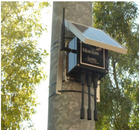
Deployed Sensor Node with solar power
