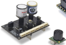
Gas-Noise-Temp.-Humidity-Dust Luminosity Sensors
